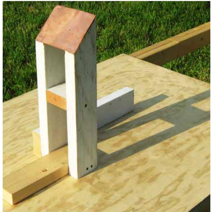
Above: A pinhole punched in a copper sheet acts as a shadow definer. In our tests, the shadow definer was able to produce an image so sharp that we could see the rod projecting from the gnomon's tip. This aid would have allowed the Egyptians to resolve a true east-west line to within a minute or so of arc.
