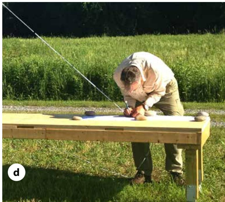
Drawing the circle. After the shadow line is established, a string is pulled from the top of the gnomon and matched with the shadow line on one side of the platform (a). The length of the line is then fixed and pulled over to the other side of the platform (b and c). The string is matched to the line there (d). The two points where the string and the line intersect should run straight east-west. Photos by Becky Dash.
